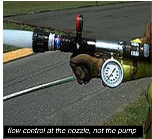
*flow control at the nozzle, not the pump*
